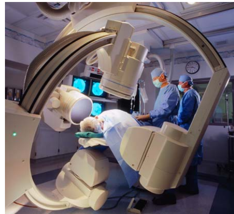
Figure 2. A fluoroscopic C-arm is an arc-shaped piece of equipment that generates x-rays from one side and photographs them on the other side.
